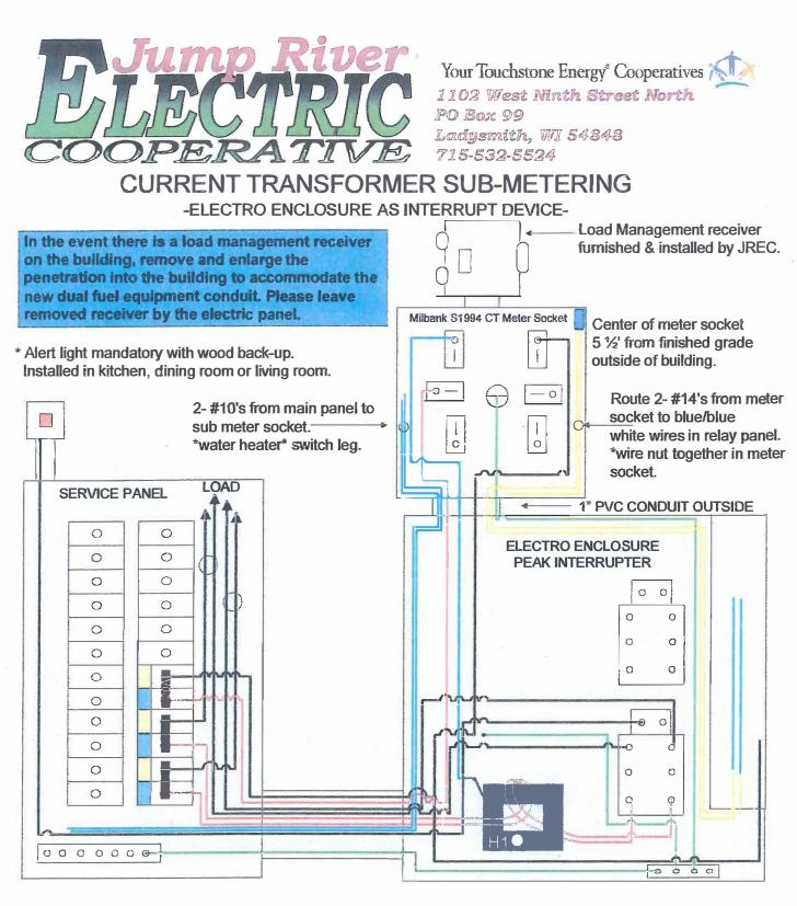
Run 2 - #10's, 2 - #14's, 6 - #12's (black, blue, green, red & 2 whites) from service panel to meter socket through 1" conduit. Leave 3' tails at each end coiled up in meter socket and panel, that are not terminated.
